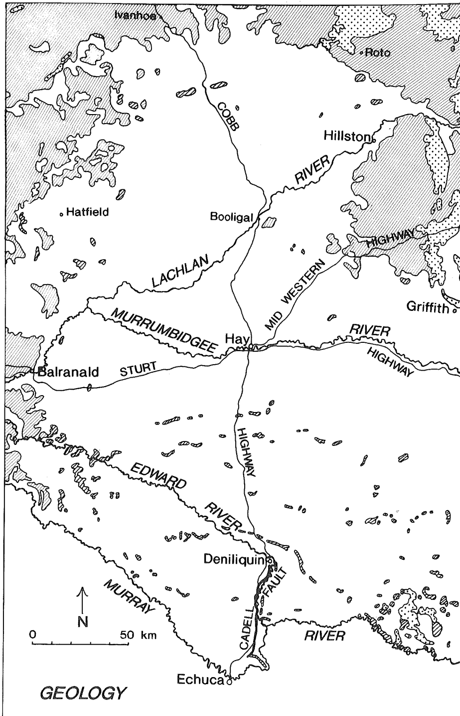
Figure 3. The geology of the mapped area. White unhatched areas indicate flat, alluvial and lacustrine deposits of clay, silt, sand and gravel. Hatched areas are largely aeolian, flat to gently undulating plains and dunes of red and red-brown clayey sands and loams. Spotted areas are sandstone-conglomerate sediments (slate and granite in the far south-east). Based on Goldberg and West (1968) and Offenbergh (1969).
